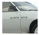
The "Manta GT/E" on either side of the car with one word on the door and the other on the wing. These fit just above the swage line. The remaining GT/E's go on the front lower airdam and the bootlid.
